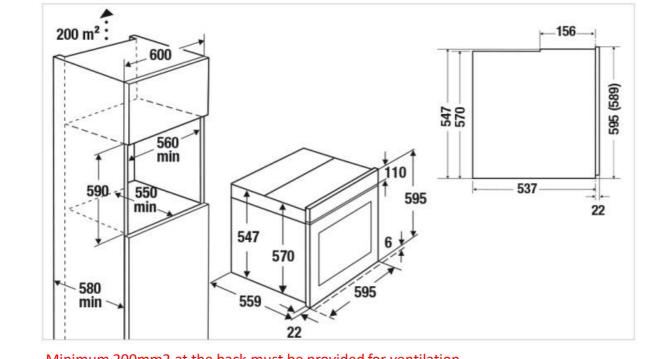
Minimum 200mm2 at the back must be provided for ventilation.
